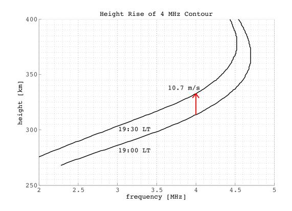
*Figure 4: The height-rise with time of the 4 MHz contour between 19:00 and 19:30 LT at Jicamarca on October 12, 2009, resulting in an inferred upward drift of 10.7 m/s.*
