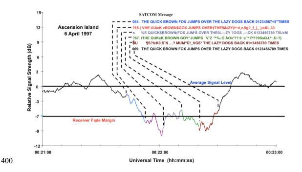
*Figure 1: A real-world example of SATCOM effects from an AFRL campaign in 1997. During periods of scintillation, the received message at Ascension Island was garbled.*
